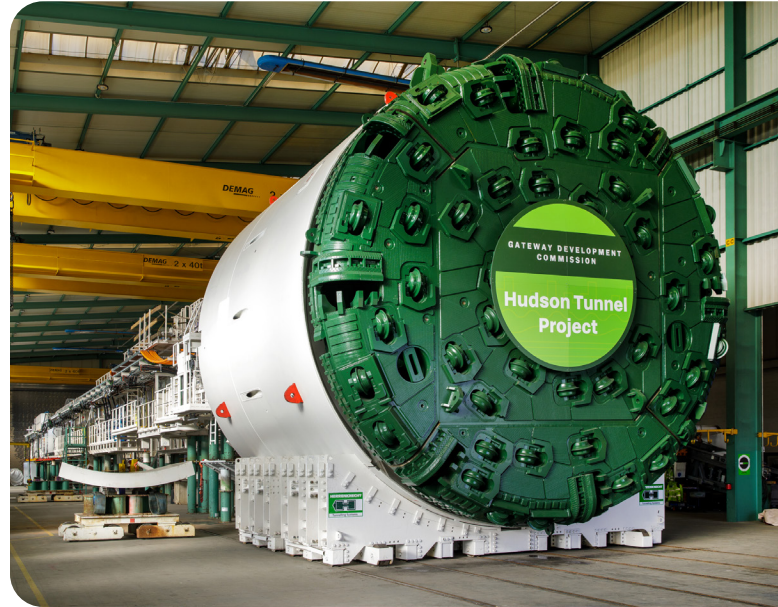
Tunnel Boring Machines will dig the tunnel section that stretches from New Jersey to the edge of Manhattan.
