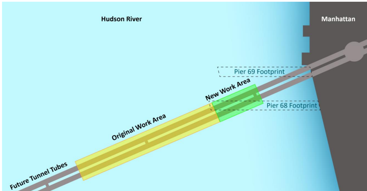
Map of the original HRGS work area and additional work area added by the change order.
