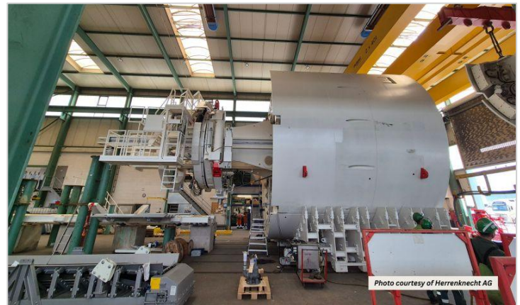
The shield for one of the TBMs that will build the new tunnel.
