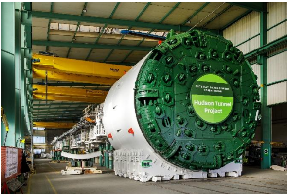
TBM S-1432 assembled at the factory for testing.
