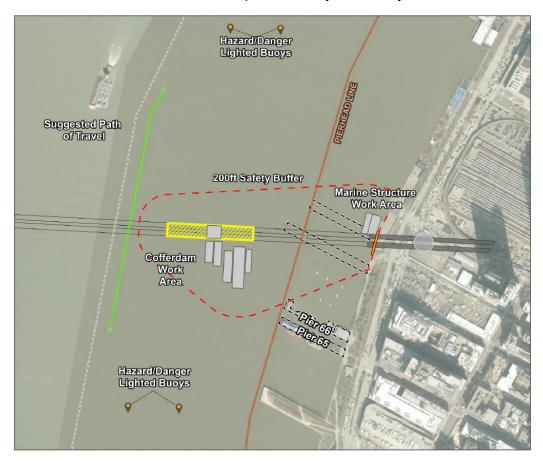
In addition to the ongoing Hudson River Ground Stabilization cofferdam operation, and as part of the Manhattan Tunnel project, GDC's contractor will begin installing marine temporary structures to hold equipment that will stabilize the ground underneath the Hudson River.
