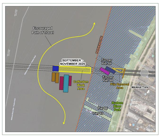
The Hudson River Ground Stabilization (HRGS) project will fortify a section of the riverbed to enable tunnel boring machine operations for the future Hudson River Tunnel.
