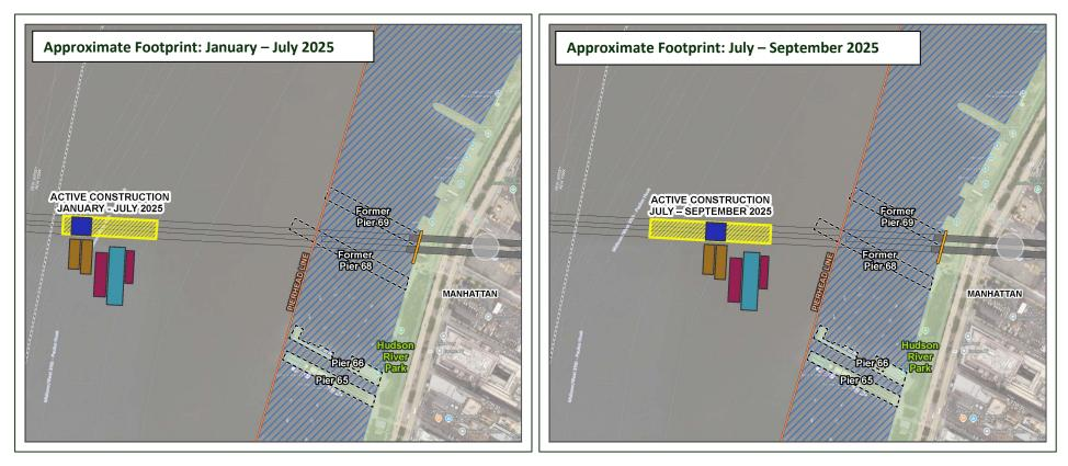
The Hudson River Ground Stabilization (HRGS) project will fortify a section of the riverbed to enable tunnel boring machine operations for the future Hudson River Tunnel.
