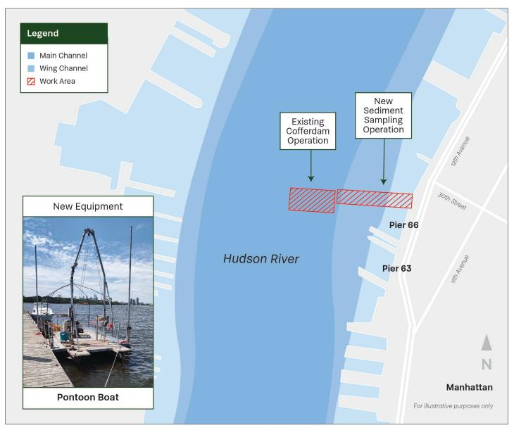
The Hudson River Ground Stabilization (HRGS) project will fortify a section of the riverbed to enable tunnel boring machine operations for the future Hudson River Tunnel.
